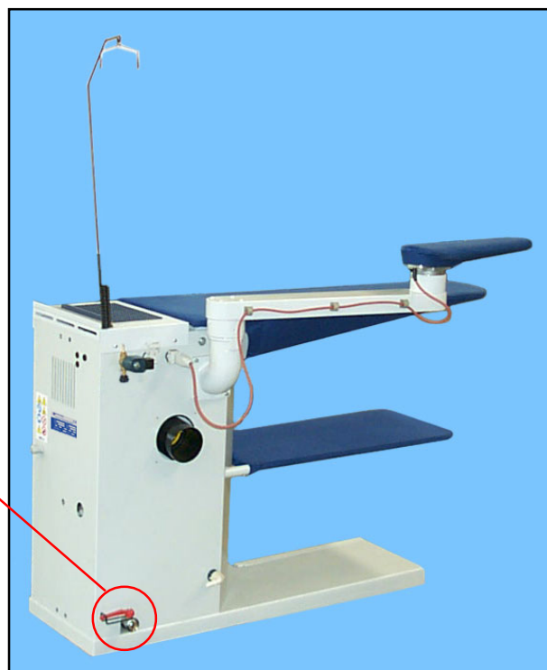
Figure chap. 10.2.1 "Discharge tap"
